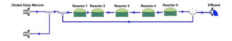
Average values of COD, Total Kjeldahl nitrogen (TKN), alkalinity, total phosphorous (TP), pH of were the chosen parameters for this study. In the model, the digester HRT was set up to be 30 days which is the value of the pilot experiments. 3.2Model calibration methods
