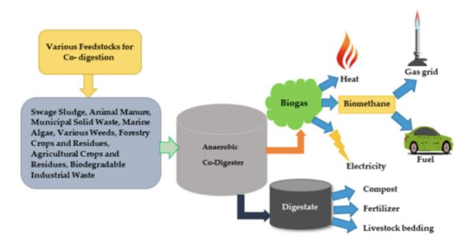
In the last few years, anaerobic co-digestion (AnCoD) has gained acceptance due to its enhancement of conservative AD technology and also due to its economic sustainability, improved methane yields, the capability to ease the existing shortcomings from mono-digestion which bring about infectivity.
